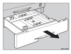
2 Open the guide in the duplex tray as shown in the illustration, and then remove the misfed paper.
